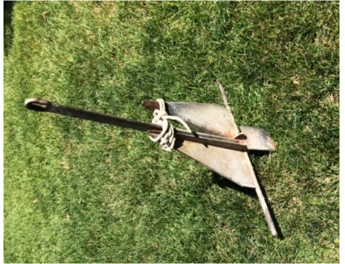
Danforth 13# anchor with 15" flukes for boats 21'-32'
