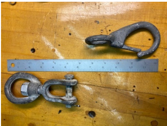
6" anchor swivel, galvanized snap hook
