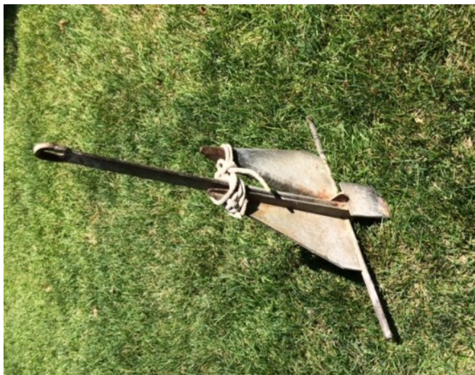
Danforth 13# anchor with 15" flukes for boats 21'-32'
