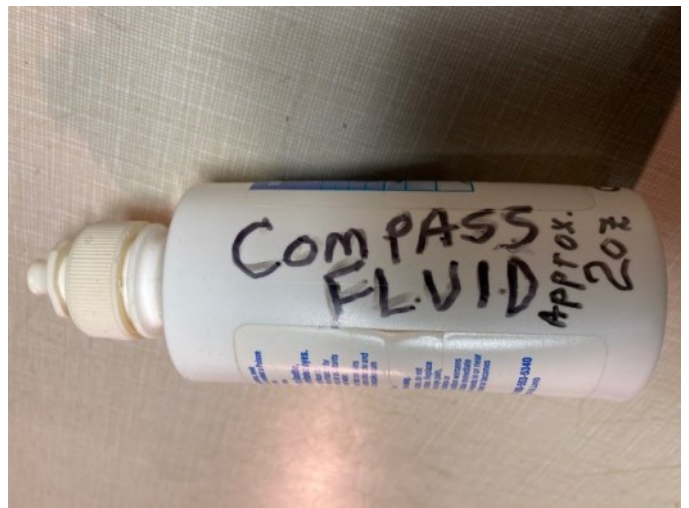
Edson compass fluid - approximately 2 oz. (used to remove air bubble in compass)
