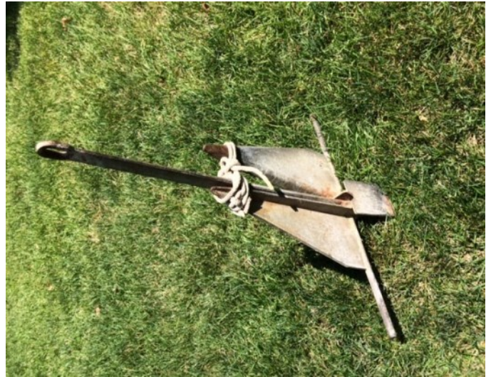
Danforth 13# anchor with 15" flukes for boats 21'-32'
