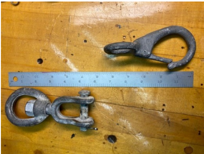
6" anchor swivel, galvanized snap hook
